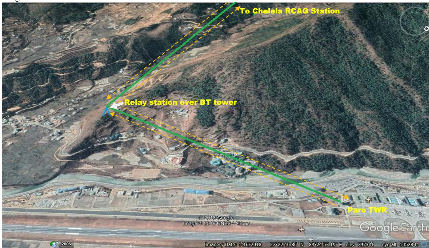
UHF links between Paro Tower – Chelela via relay station over the BT tower at Woochu ridge
